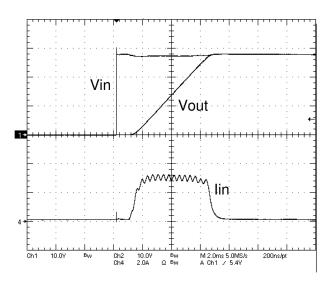
**Figure 6** – Vin, Vout, lin during turn-on at 28V, Cout=500μF
