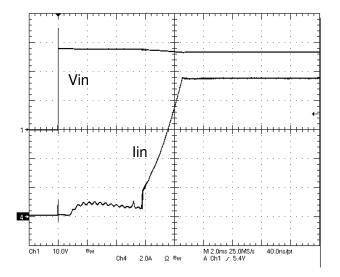
Figure 4 – Vin, lin during turn-on at 28V with DVME28, Cout=100 $\mu$ F and 2x DVFL2800S at full load
