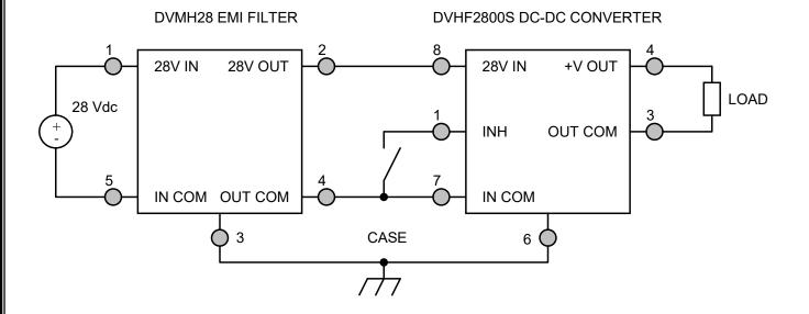
Figure 3 – DVMH28 EMI Filter Hookup with Single Converter
