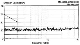
Figure 9 – MIL-STD-461C Two DVHF2800S's With DVMH28 EMI Filter
