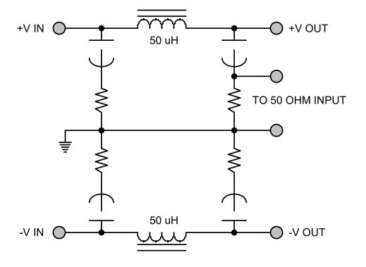
Figure 6 – MIL-STD-461D Measurement Method (LISN)
