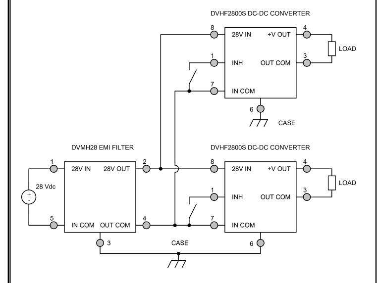
Figure 4 – DVMH28 EMI Filter Hookup with Two Converters
