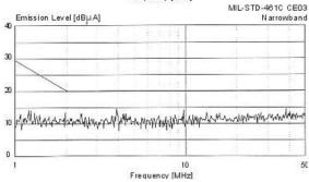
Figure 8 – MIL-STD-461C DVHF2800D With DVMH28 EMI Filter
