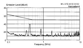
Figure 10 – MIL-STD-461D DVHF2800S With DVMH28 EMI Filter
