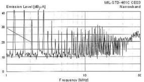
Figure 7 – MIL-STD-461C DVHF2800D Without EMI Filter
