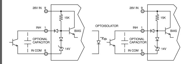
**Figure 4** – Internal Inhibit Circuit and Recommended Drive (Shown with optional capacitor for turn-on delay)
