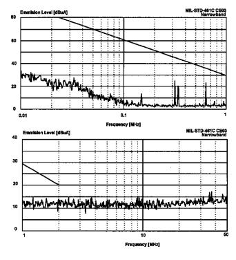
Figure 12 - DVGF+2800T with EMI Filter
