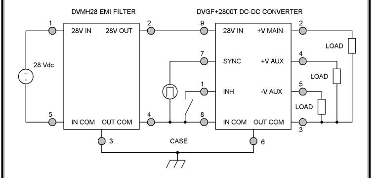
Figure 6 – Converter with EMI Filter
