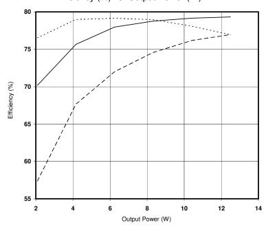
Figure 8 – DVGF+283R315T Efficiency (%) vs. Output Power (W)
