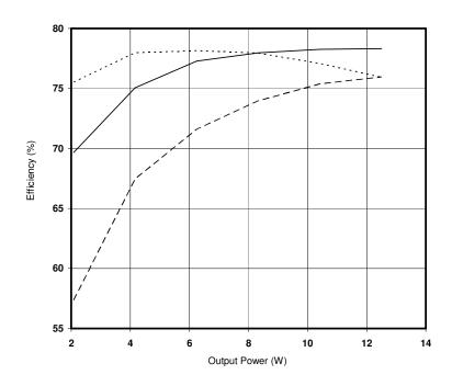
Figure 7 – DVGF+283R312T Efficiency (%) vs. Output Power (W)
