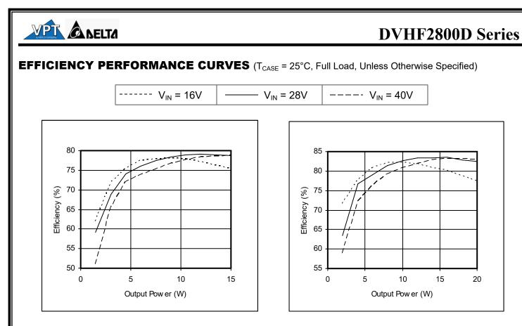
**Figure 7** – DVHF2805D Efficiency (%) vs. Output Power (W)
