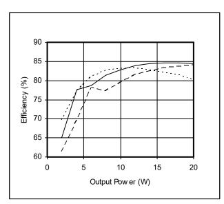
**Figure 9** – DVHF2815D Efficiency (%) vs. Output Power (W)
