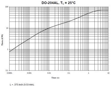
$R_{BJL} = 70^{\circ}$ C/W.  $Z_{BJX} = 10^{\circ}$ C/W maximum at t<sub>H</sub> = 10ms.
