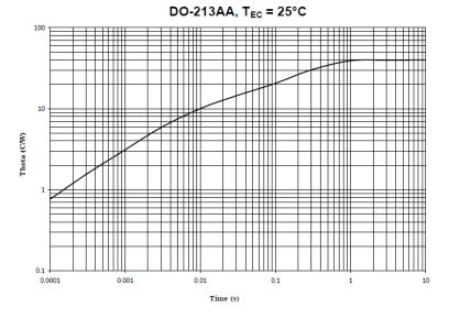
$<sup>\</sup>label{eq:generalized_linear} \begin{array}{l} L=0.\\ R_{\text{RJEC}}=40^{\circ}\text{C/W}.\\ Z_{\text{RJX}}=10^{\circ}\text{C/W} \text{ maximum at } t_{\text{H}}=10\text{ms}. \end{array}$
