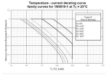
Sinewave operation 50 percent duty cycle  $R_{\text{BJL}} = 70^{\circ}\text{C/W}$
