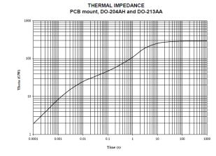
NOTE: Thermal resistance = 300°C/W. Maximum power rating = 400 mW at T<sub>A</sub> = 55°C.
